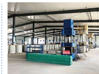
8. 2000T Four-Column Hydraulic Press Nominal pressure of 2000KN ejector pressure Can produce SMC parts up to 1.8x3.5m
