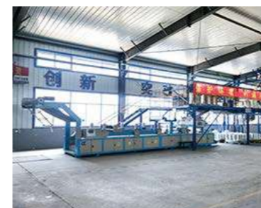
7. SMC Sheet Production Line Multi-Screw SMC Sheet Machine Fully automated dosing system to ensure dosing accuracy
