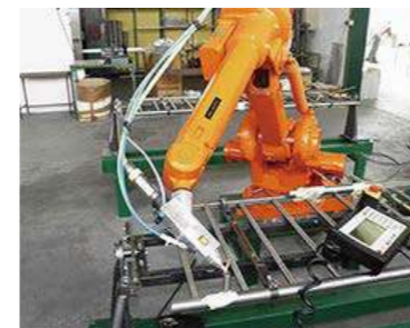
4. Welding Robot Six-Axis Welding Robot with ABB Mechanical Arm Automatic weld seam recognition and tracking
