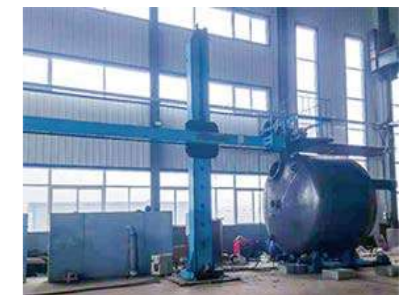
6. Cross-arm Automatic Welding Equipment Submerged Arc Automatic Cantilever Welding Capable of welding \phi 500\text{-}\phi 5000 ring seams
